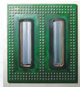
Die-down BGA sample after rotation and decapsulation of glob 2.
