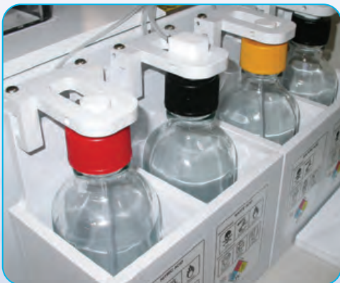
Bottle cap detail showing cap assembly integral to bottle box containment unit.
