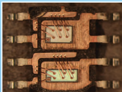
SOIC-8 sample with copper wires, etched with mixed-acid ratio; also showing complete second bond
