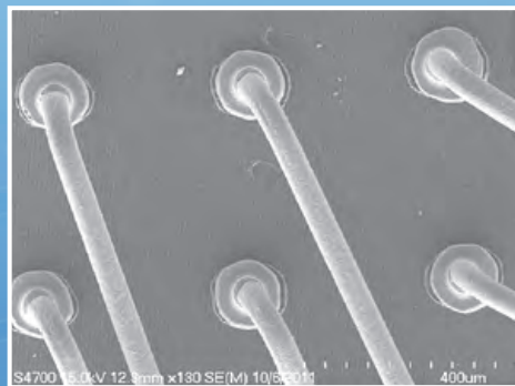
SOIC-8 sample with copper wires, showing complete integrity of wire bonds after decapsulation
